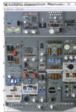
*Note: if you close the OVH737FWD test windows returning to the TEST\_OH main window, when you open it again, all the switch positions will not be displayed. To synchronize the screen click on "Reset" button on the menu bar.*
